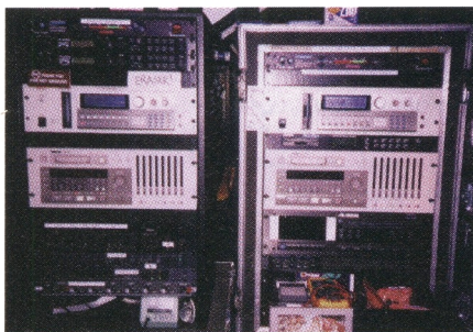
The Nine Inch Nails power station. Left rack: Furman PL8 power module, two Alesis D4s, Akai S3000, Tascam DA-88, Yamaha MV-802 mixer, and audio modules from Toa, Crest, and Rane. Right rack: Furman PL8 power module, Alesis ADAT, and Alesis MicroVerb.
